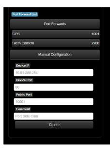
To set port forwarding enter **Device IP**, **Device Port**, **Public Port** and **Comment**. Click **Create** to add it to Port Forward List. This feature is useful when you want to set port forward for device that has static IP address and is not listed on DHCP Client List (chapter "2.14. VESSEL NETWORK - ADVANCED SETUP" on page 32).
