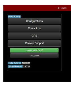
Click on **Connect** button to connect Yacht Router to Support Network. Once it is successfully connected button will go green and **Connected ID** number will appear.
