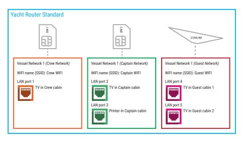
Here you can see schematic example of Vessel Network setup on Yacht Router Standard. Device is transmitting three Vessel Networks WIFI (Crew WIFI, Captain WIFI, Guest WIFI). Each Vessel Network is connected to different Internet source (SIM 1, SIM 2, Starlink). LAN ports on Yacht Router device are set to be part of different Vessel Networks where LAN port 1 is part of Crew Network, LAN port 2 and 3 part of CAptain Network and LAN port 4 and 5 part of Guest Network.
